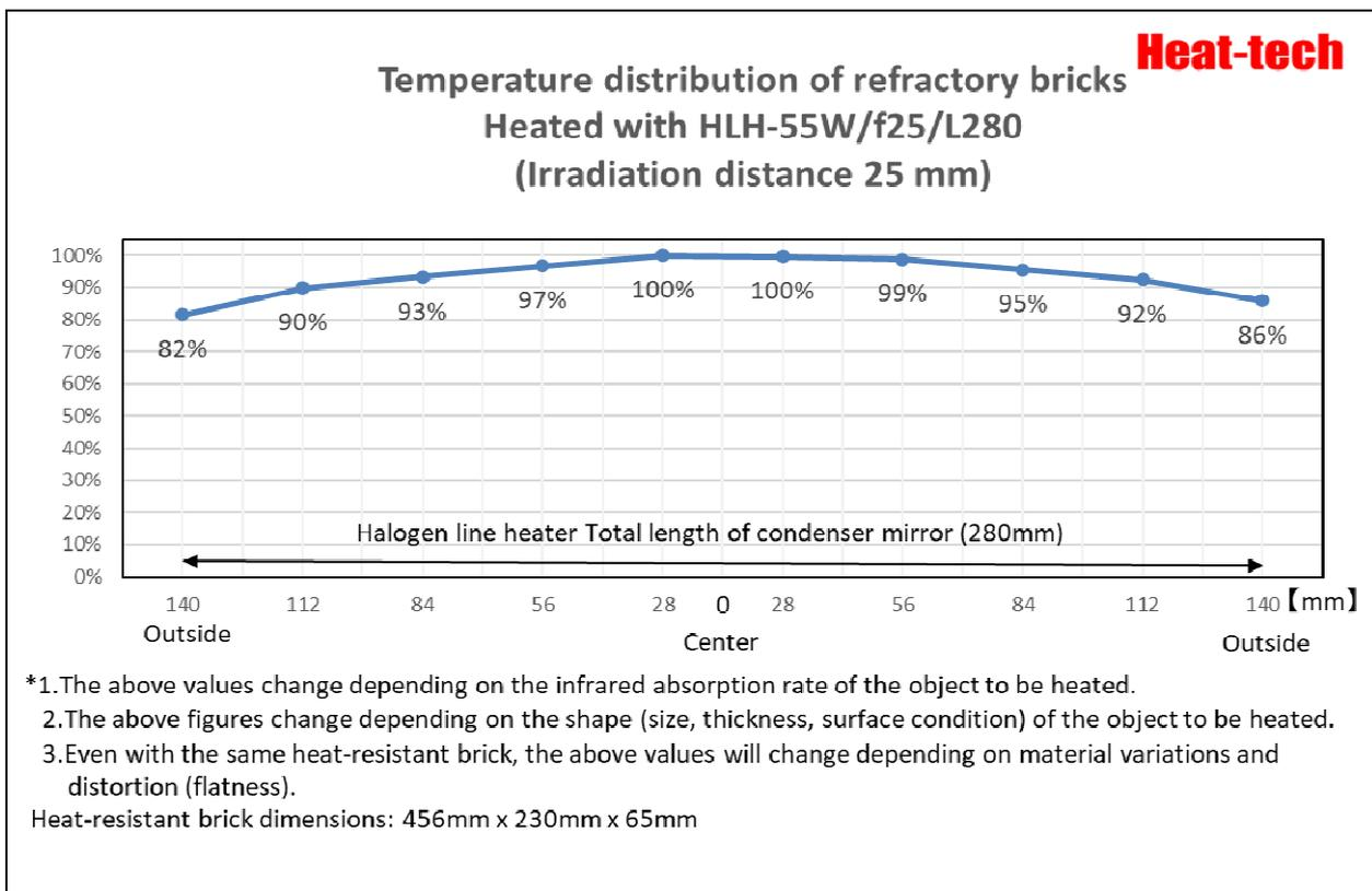
From the thermal image, divide the 280 mm area of the condenser mirror of the halogen line heater into 10 areas, divide the maximum temperature of each divided area by the maximum temperature of the entire area, and quantify the temperature distribution of the heat-resistant bricks.
