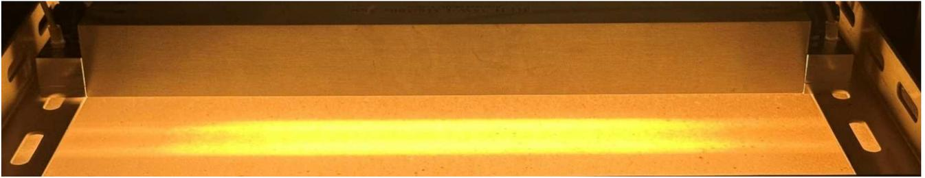
HLH-35W/f $\infty$ /L316 irradiates refractory bricks from a distance of 30mm.
