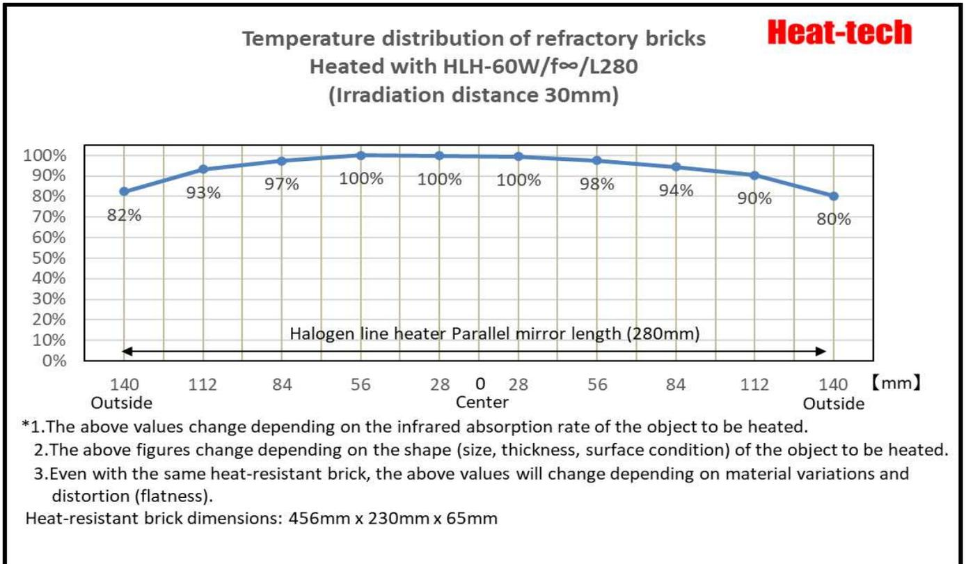
From the thermal image, divide the 280 mm area of the condenser mirror of the halogen line heater into 10 areas, divide the maximum temperature of each divided area by the maximum temperature of the entire area, and quantify the temperature distribution of the heat-resistant bricks.
