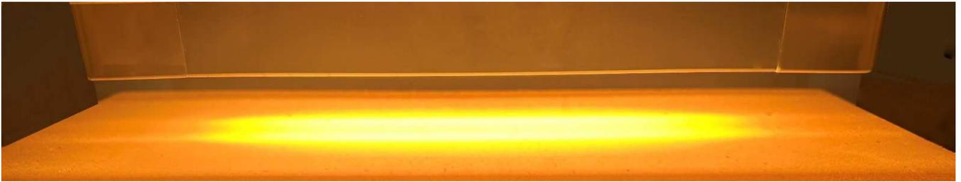
HLH-50W/f $\infty$ /L280 irradiates refractory bricks at a distance of 30mm.
