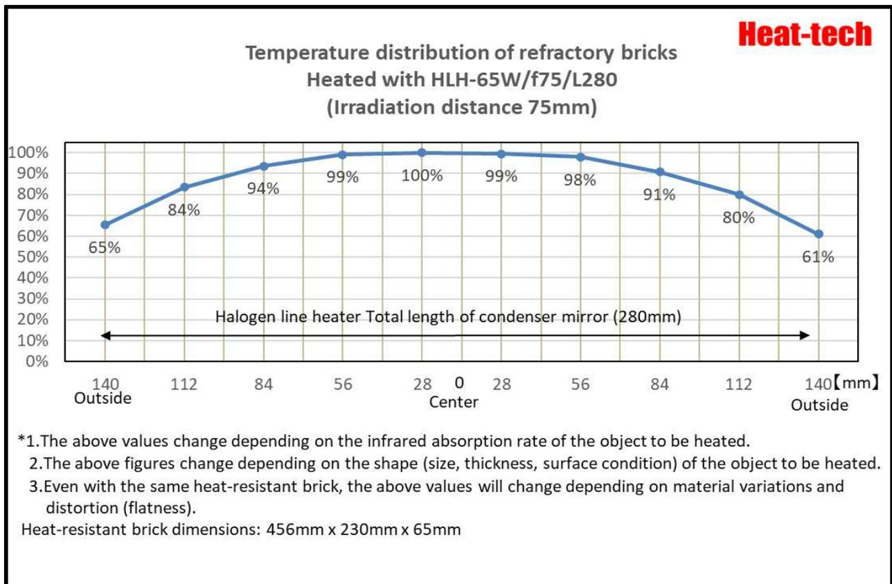
From the thermal image, divide the 280 mm area of the condenser mirror of the halogen line heater into 10 areas, divide the maximum temperature of each divided area by the maximum temperature of the entire area, and quantify the temperature distribution of the heat-resistant bricks.
