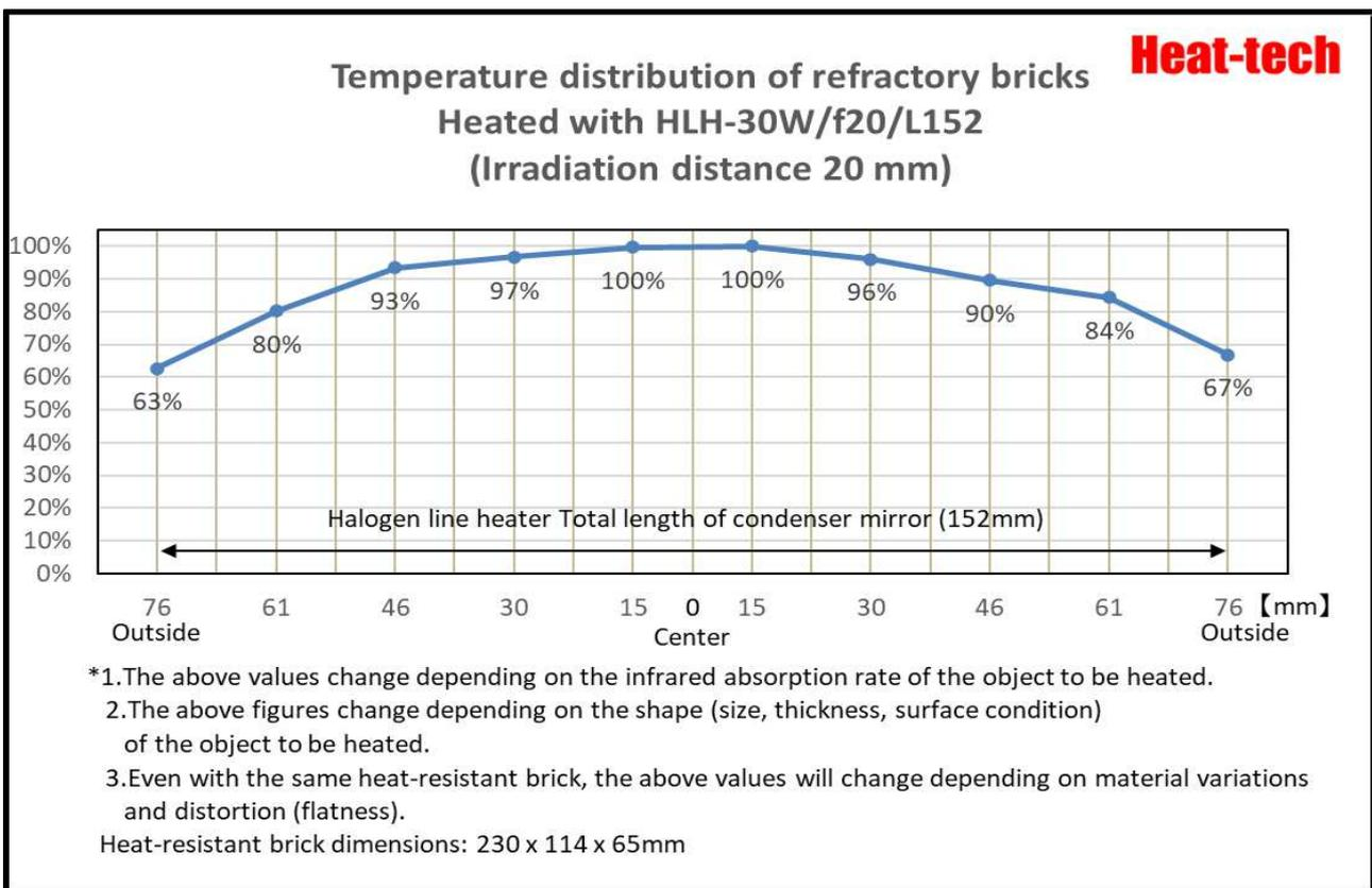
From the thermal image, divide the 152 mm area of the condenser mirror of the halogen line heater into 10 areas, divide the maximum temperature of each divided area by the maximum temperature of the entire area, and quantify the temperature distribution of the heat-resistant bricks.
