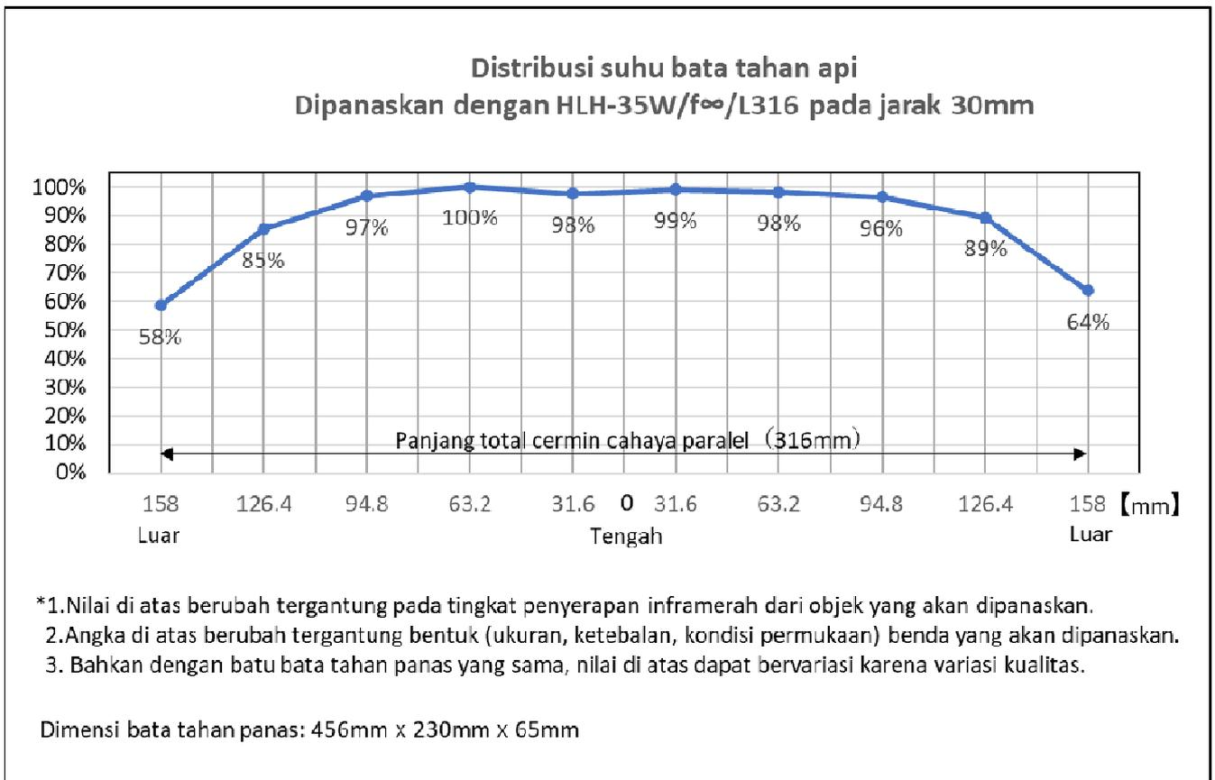
From the thermal image, divide the 316 mm area of the condenser mirror of the halogen line heater into 10 areas, divide the maximum temperature of each divided area by the maximum temperature of the entire area, and quantify the temperature distribution of the heat-resistant bricks.
