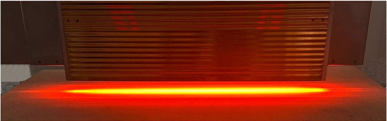
HLH-55W/f25/L280 from a rated focal length of 25mm irradiates firebricks.
