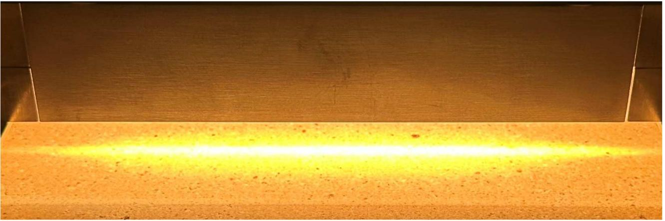
Refractory bricks are irradiated with HLH-30W/f30/L152 from a rated distance of 20mm.
