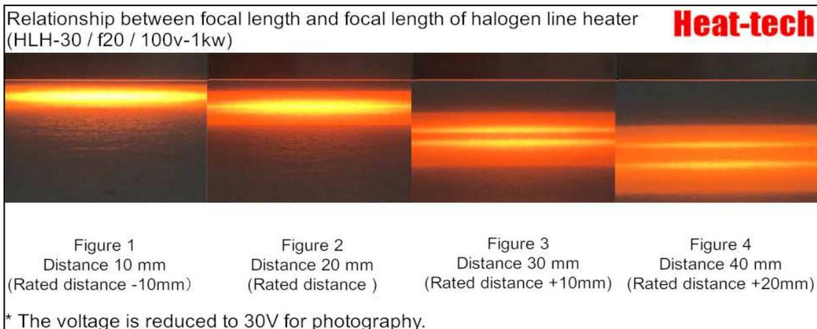
If HLH-30 is separated from a focal length (20mm), it can also perform heating which gave width. Irradiation intensity is even, but the temperature of the center of the higher heat of the peripheral portion is run away.
